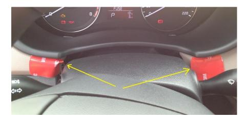
BEFORE STARTING THE DISASSEMBLY PROCESS, APPLY THE 3M PROTECTIVE TAPE, WHICH COMES IN THE BOX, ONTO THE LOWER RIGHT AND LEFT-HAND SIDE CORNERS AS SHOWN IN THE FIGURE IN ORDER NOT TO HARM THE LEATHER COVER WHILE REMOVING THE
