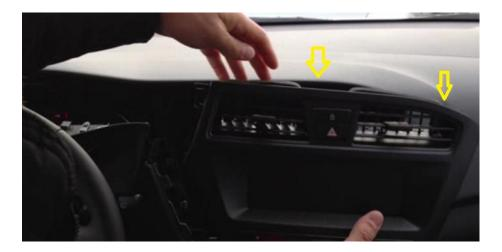
REMOVE BY PULLING AND WITHOUT DAMAGING THE SOCKET CONNECTORS AT THE BACK OF THE VENTILATION FRAME.
