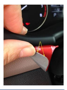
ONCE THE ASSEMBLY PROCESS IS COMPLETE, REMOVE THE 2 PIECES OF 3M PROTECTIVE TAPE THAT YOU HAVE APPLIED BEFORE.
