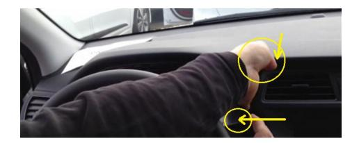
START TO SEPARATE THE VENTILATION FRAME EDGES FROM THE TABS CAREFULLY.
