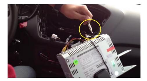
CAUTIOUSLY MOUNT THE SOCKETS, WHICH ARE ON THE VEHICLE SIDE, ONTO THE BACK SIDE OF THE MULTIMEDIA DEVICE.
