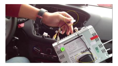
HOLD THE DAIICHI DVD MULTIMEDIA DEVICE AND FIX THE GPS ANTENNA ONTO THE DEVICE USING THE ADHESIVE TAPE AT THE BACK.
