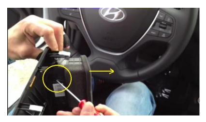
SEPARATE THE VENTILATION GRID LOCATED ON THE FRAME YOU HAVE REMOVED FROM THE CONNECTING
