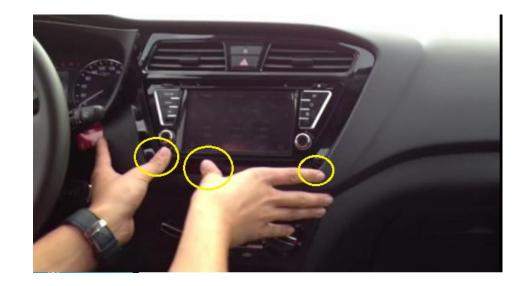
COMPLETE THE CHECKING PROCESS BY CHECKING THE EDGES OF THE FRAME WITH YOUR FINGERS. MAKE SURE THAT IT IS SEATED.
