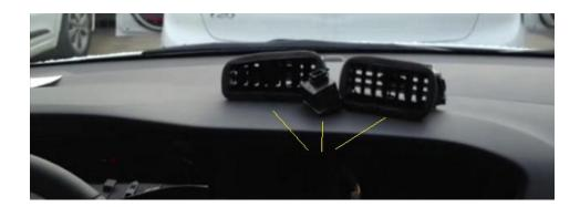
PLACE THE 2 GRIDS AND THE FLASHER THAT HAVE COME OUT OF THE FRAME ONTO THE GLOVE COMPARTMENT.
