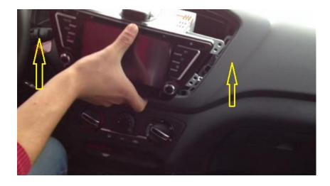
PLACE THE MULTIMEDIA DEVICE IN ITS HOUSING ON THE VEHICLE SIDE CAREFULLY.
