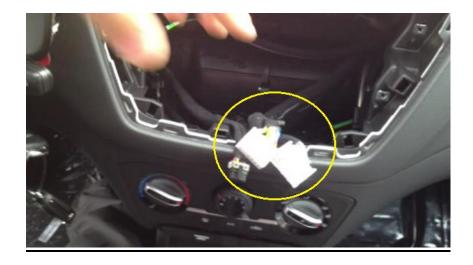
THE SOCKETS HAVE BEEN REMOVED FROM THE FRAME, HOUSING IS FREE.
