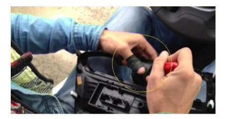
UNSCREW THE FLASHER IN THE FRAME WITH THE HELP OF A SCREWDRIVER.
