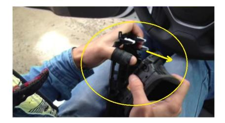
REMOVE THE VENTILATION GRIDS FROM THE FRAME.
