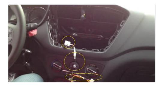
HOLD THE VEHICLE'S PARKING BRAKE CABLE WHICH YOU HAVE BROUGHT TO THE BACK OF THE RADIO HOUSING AND THE YELLOW CABLE WHICH HAS COME OUT OF THE DAIICHI BOX AND IS SHOWN WITH <u>NUMBER 6</u> IN THE FIRST FIGURE. INTEGRATE THIS CABLE WITH THE PARKING BRAKE CABLE OF THE VEHICLE.
