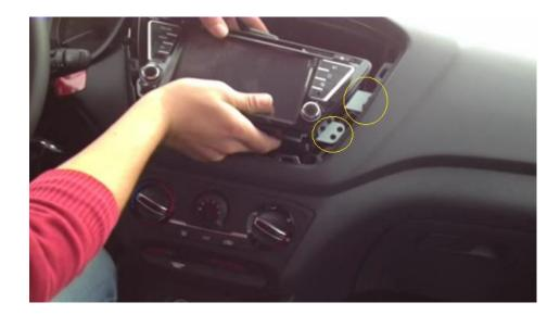
BRING THE MULTIMEDIA DEVICE INTO ALIGNMENT WITH THE SCREW HOLES ON THE VEHICLE SIDE.
